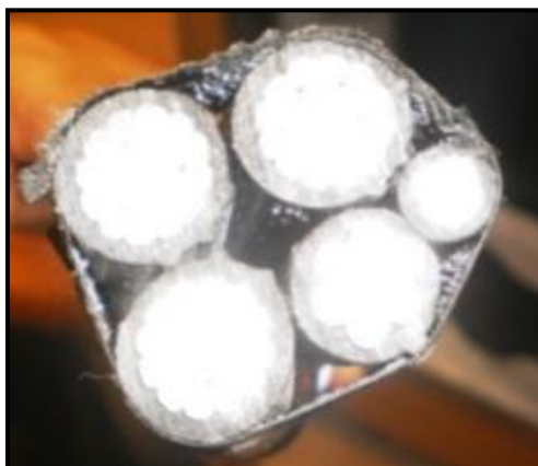
Figure 16. Cross-section view of ABC (b)
