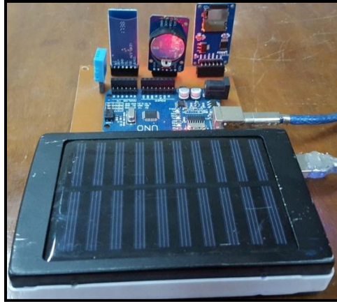
Figure 8. Data Logger Hardware (b) with Solar Panel
